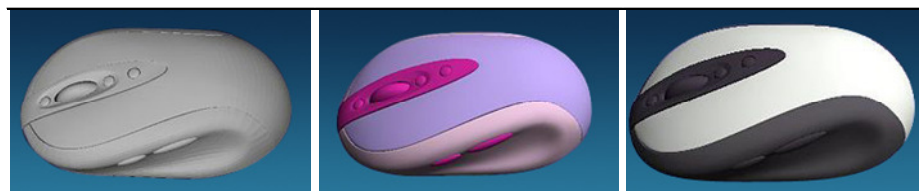
Figure 1: Effect of geometric modelling at different stages: no colour (left), random colouring (middle) and coloured according to colour design tool (right).
