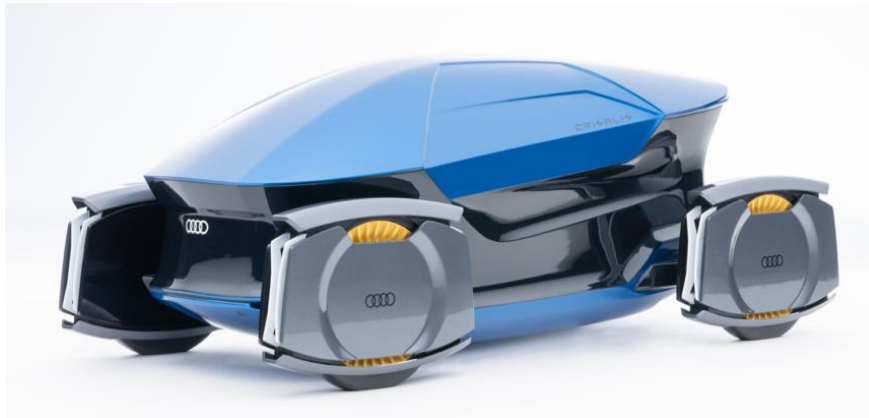
Figure 4: 1:4 scale model created with a CNC machine and painted with the first CMF proposal represented in Figure 3. Audi Crialis by F. Batavia, J.P. Bruni, E. Trabattoni, P.E. Tranchellini (June 2019).
