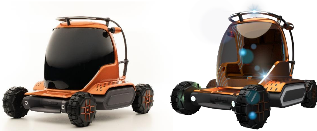
Figure 7: GoPro Chios by E. Campinotti, R. Gallo, R. Nagaraj, S. Toninato (July 2021). On the left is the physical model in the 1:10 scale, on the right is a rendered image: both representations are from a 3D digital model done by students.
