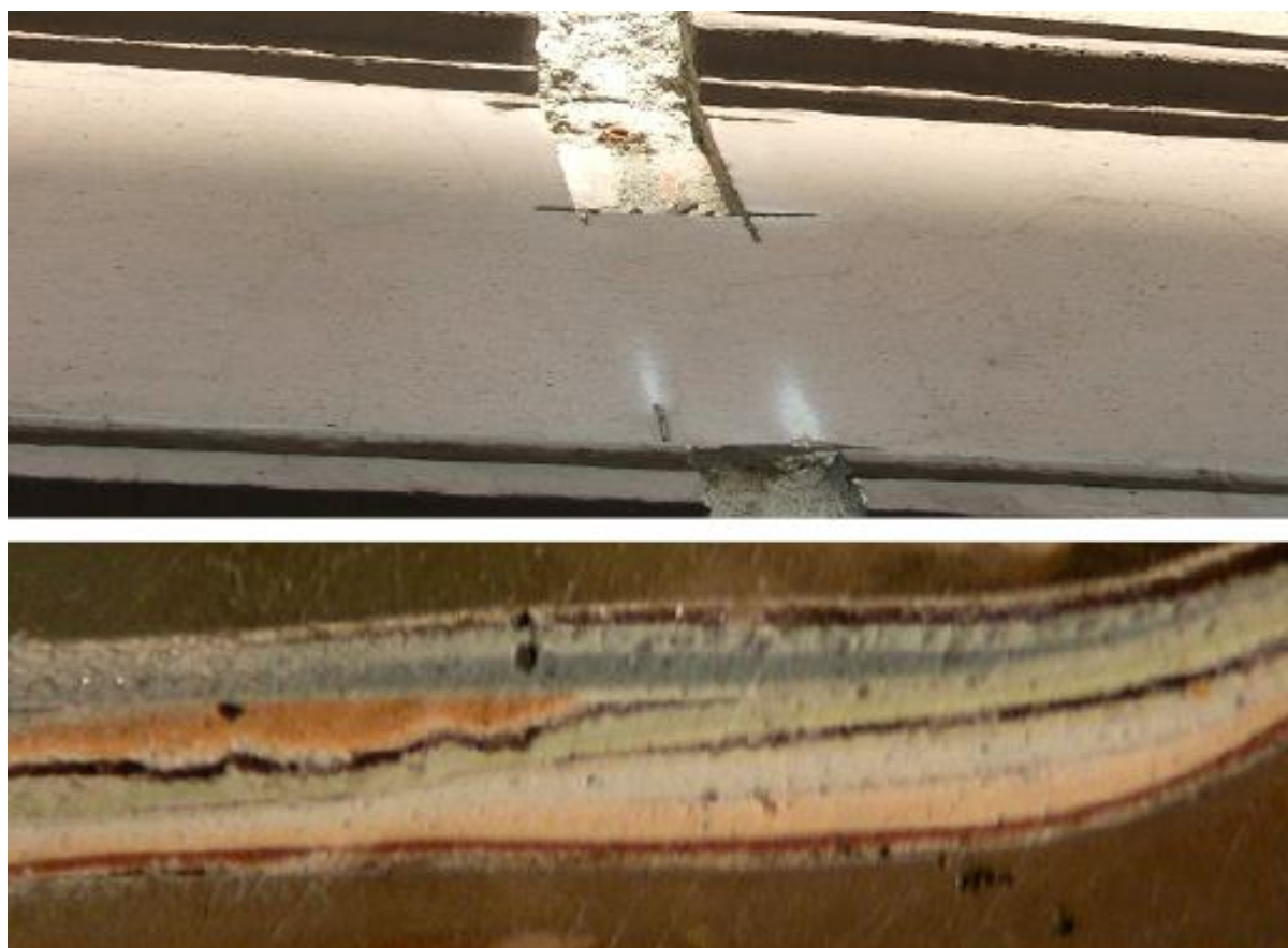
Figure 6: The difference in visibility of the sequence of plaster and paint layers on site and under the microscope. By the author (upper picture), courtesy by Barbara Kubisa (bottom picture).
