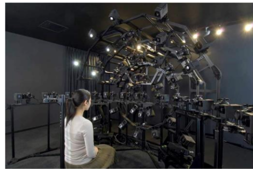
Figure 1: Multi-angle Image Capturing System.
