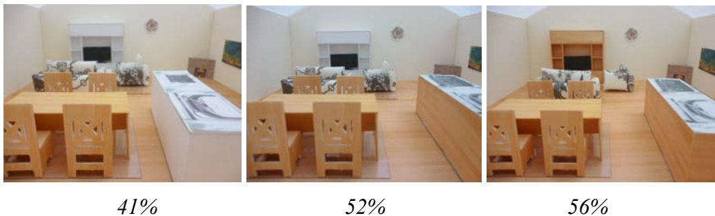
Figure 1: Examples of the scale model with different proportions of the wooden finish area
