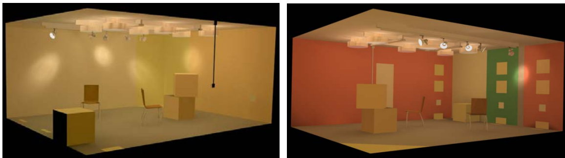
Figure 1A,B: The reference room, designed to show clear examples of how simultaneous contrast phenomena and reflections cause different appearances.
