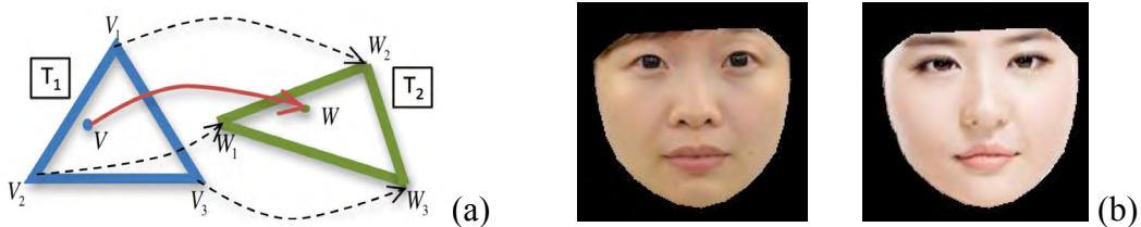
Figure 5: (a) Triangulation and interpolation, (b) Images before and after affine transformation
