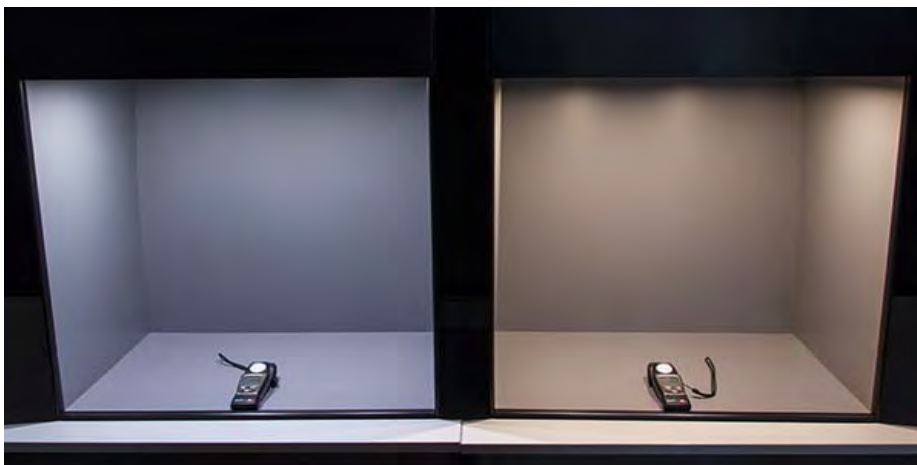
Figure 3: Two lighting cabinets illuminated by LED light sources of different CCT.
