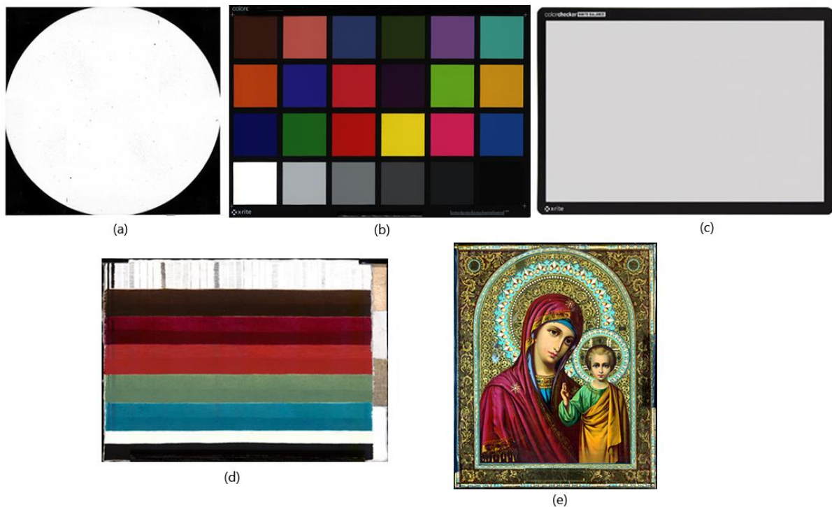
Figure 1. RRT test objects (a) Spectralon reference (b) ColorChecker Classic (c) White balance (d) Painted panel (e) Icon
