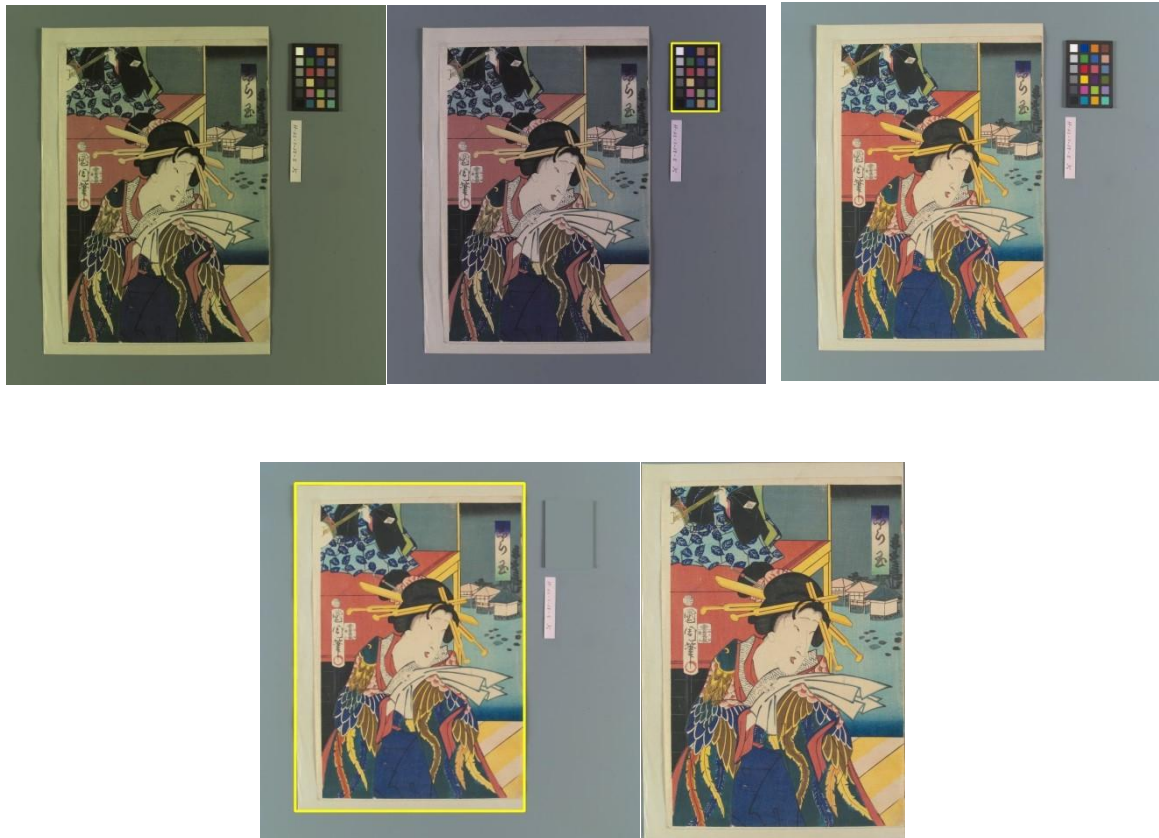
Figure 3. Original Nishiki-e image (upper-left), detection of color chart (upper-middle), color-corrected image (upper-right), detection of Nishiki-e picture (lower-left), and extracted Nishiki-e picture (lower-right).
