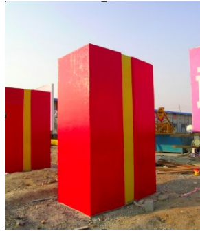
Figure 9. Life-size concrete model painted with the candidate Chinese RED on site.
