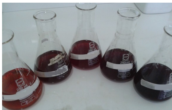
Figure 3. Second optimization. From left to right: Medium5-1, Medium 5-2 Medium 5-3, Middle 5-4 East5-5. The Medium 5-2 that had an average salt concentration and showed higher levels of absorbance and color was selected.
