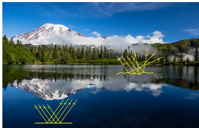
Figure 1. A mirror image, produced by regular reflection (bottom left), and a blurred image, produced by diffuse reflection (middle right).
