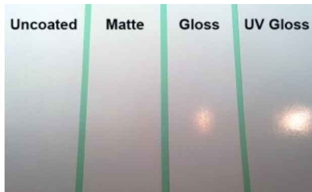
Figure 3. A series of paper surfaces with different visual appearances or cesias, showing increasing gloss from left (highly matte) to right (highly glossy). (image from The MGX Copy Blog)
