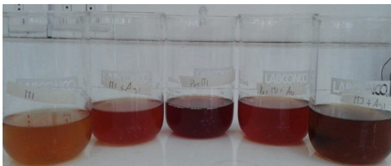
Figure 2. Optimize production of coloring pigments from Epicoccum sp. D . From left to right: Medium 1, Medium 2, Medium 3, Medium 4 Medium 5. Medium 5 was selected for its color intensity and higher absorbance values.
