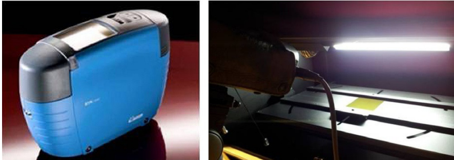
Figure 1: Left: gonio-spectrophotometer BYK-Mac; Right: Gonio-spectrophotometric system formed by the PR-650 tele-spectroradiometer and the Byko-spectra effect lighting booth.
