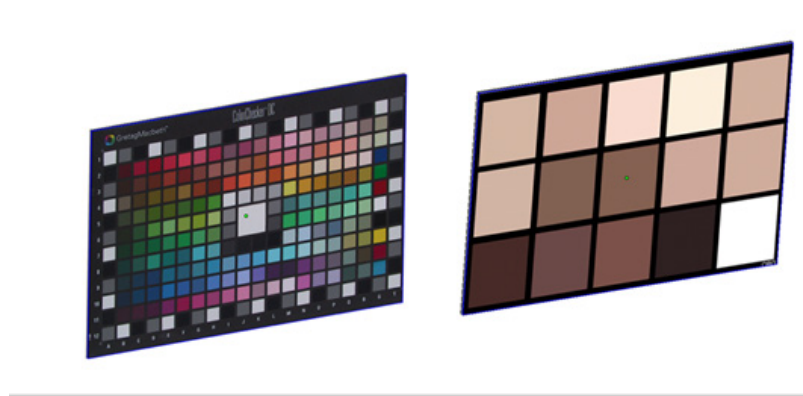
(a) Training colours (b) Testing colours Figure 2: Colour charts for 3D image reproduction.
