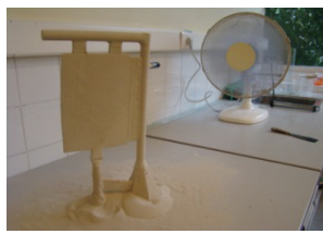
14 successive ceramic layers of increasing thickness are deposited. Drying: 4h each
