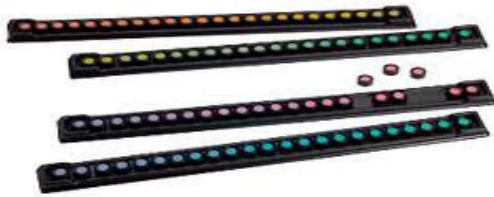
Figure 1a. FM 100 Hue test. 85 colour caps in one nuance with one fixed cap at each end, total 97. The round colour caps 11 mm diam, shall be mounted in the four test cases.
