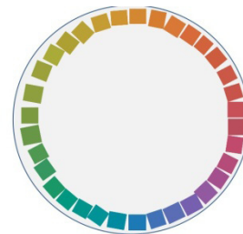
Figure 1b. The colour test used. 35 NCS colour samples on a round plate with a rim. Here test 1, the chromatic nuance S 2050.
