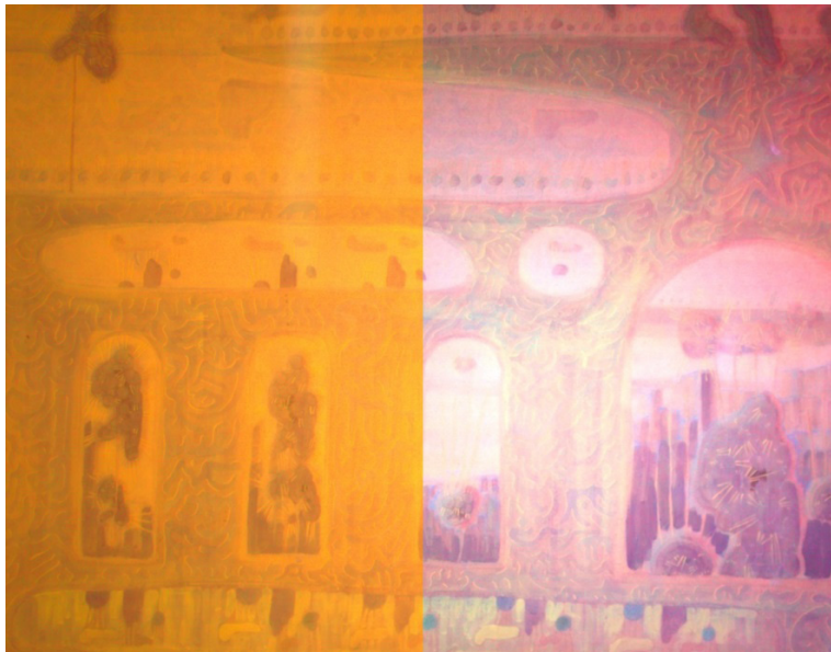
Figure 1: “Fantasy” by M. K. Čiurlionis (1908). View under original illumination by a halogen lamp (left); same painting under colour rendition engine (CCT = 6500K) with the shifted colour gamut and increased chromatic contrast (right).
