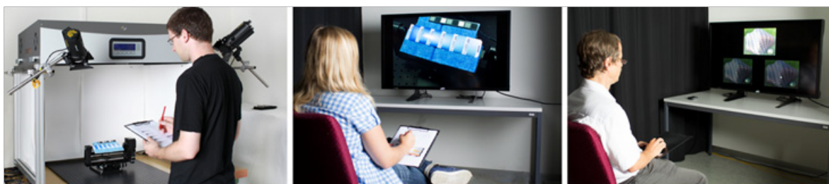
Figure 1: left - judging rotational scene in light booth, middle - judging HDR representation on HDR display, right - judging HDR and LDR images on HDR display.
