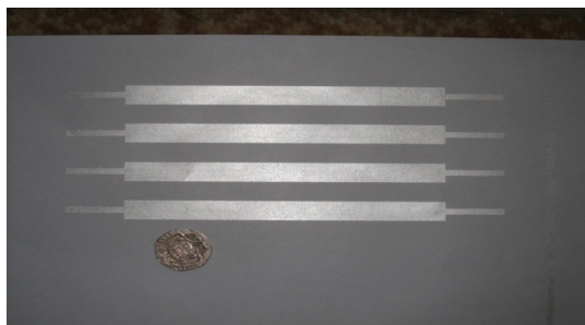
Figure 2. Silver electrodes prepared using the TacJet printing process.
