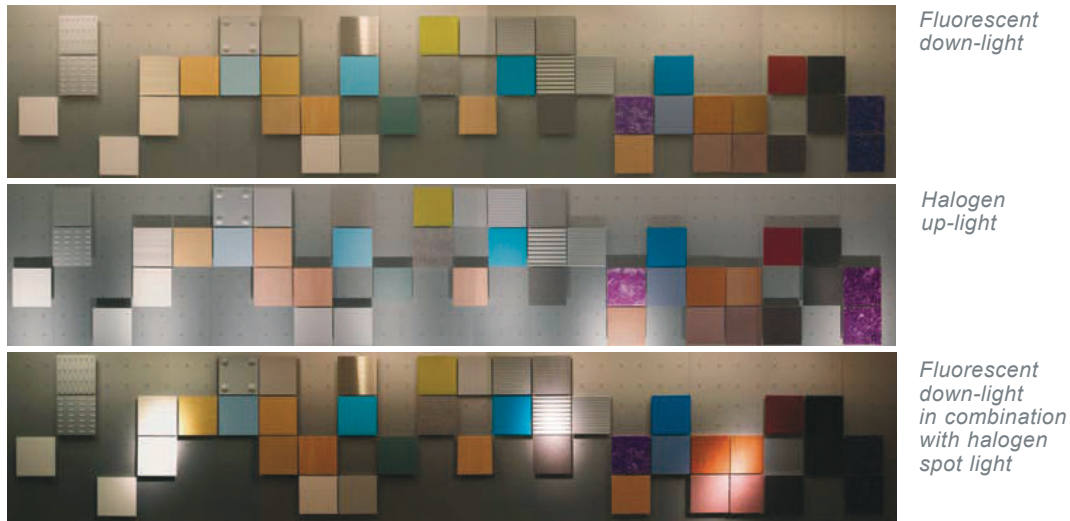
Figure 5. Material wall illuminated with fluorescent down-lights, halogen up-lights and a combination of fluorescent down-lights and halogen spots.
