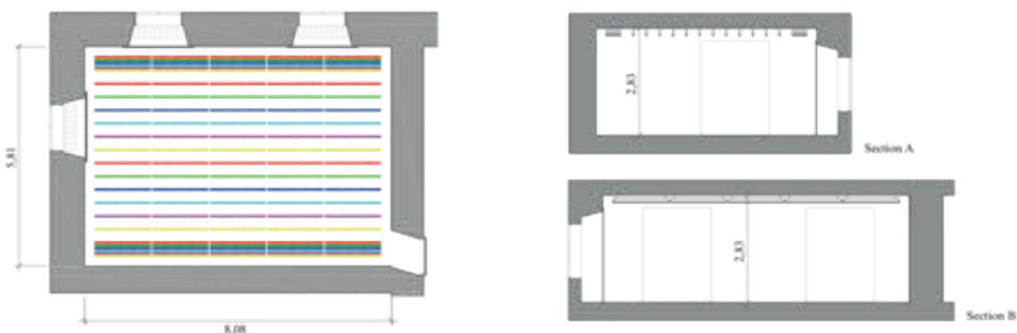
Figure 1. Spatial conditions and Lighting in plan view and two sections (A and B)
