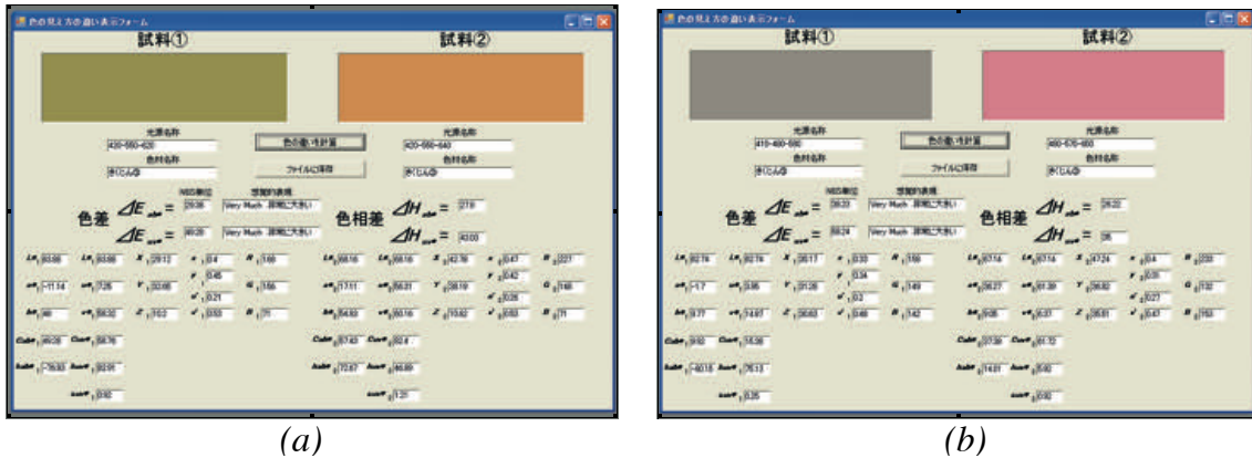
Figure 2: Result of color simulation of Japanese dye goods “Kikujin” which is originally pale green in daylight. (a): left = “Kikujin” in white light (420-550-620), right = “Kikujin” in white light (420-550-640), (b): left = “Kikujin” in white light (410-480-580), right = “Kikujin” in white light (480-570-650)
