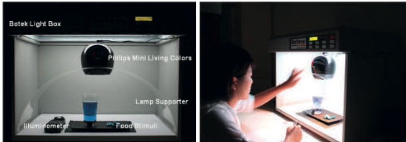
Figure 1. The setting of the empirical study: As the color varied, the illumination was varied between 300 and 600lx, a range acceptable for a dining table according to the KS A 3011 specifications.
