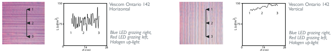
Figure 9. Photographs and measured luminance profiles for the differently oriented material samples.
