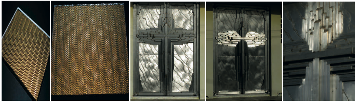
Figures 9-10. Two sheets of the same expanded metal mesh, with slight angular variation. Light to the front side (9): the upper grid only is visible. Light to the back side (10): moiré effect, with a brilliancy of leaded glass due to multiple reflections and thickness resulting from the superposed grids. – Figures 11-13. Brushed stainless steel design, Raphael Seretti, 2003-2004, door of Saint-Antoine church, Cayenne, French Guyana. The contrast results from the brushing direction, oblique on the background, parallel to the direction of the square tubes on the cross. The effect varies with the viewing point (11-12), the view angle (13) and the direction of the sun, which depends on the orientation of the wall, the latitude, the season and the hour.
