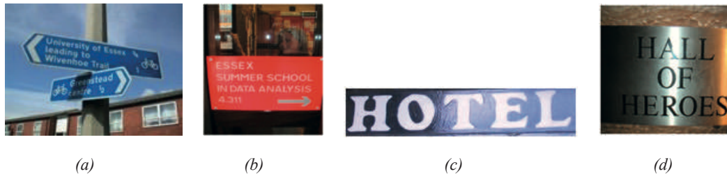
Figure 1. (a) Color changes due to shading, (b) local variation in the intensity of the illumination, (c) specularities, (d) specularities and inter-reflections.
