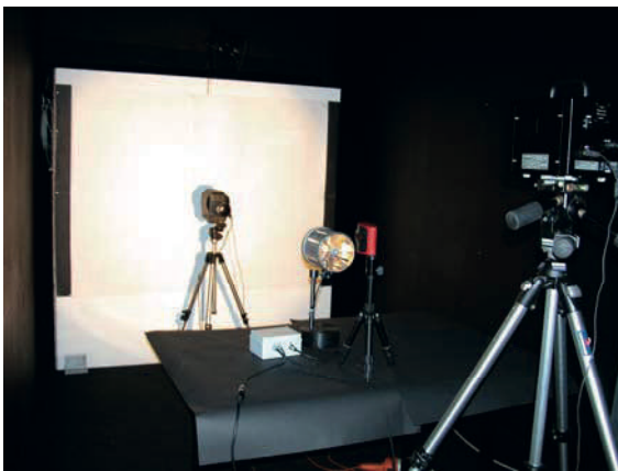
Figure 1. The measurement set-up during the calibration phase by using a spectroradiometer Spectrascan PR701.
