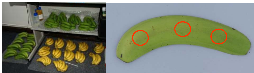
Figure 1. Left: banana samples are grouped and numbered in green (un-ripe) and yellow (ripe) colours in the laboratory; Right: measuring positions on banana skin.
