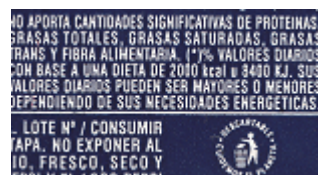
Fig.4. This printed meets Argentinian law because the uppercase has 1.8 mm height. Note that the circle is 6 mm.
