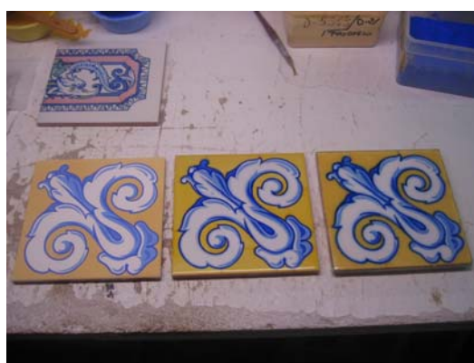
Figure 4. Glazed with tropa , before and after the firing.
