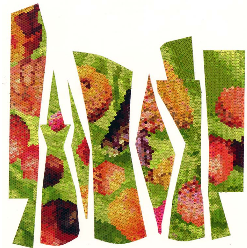
Figure 5. Final color composition, showing the distribution of everyone of the small hexagonal tiles all over the roof.
