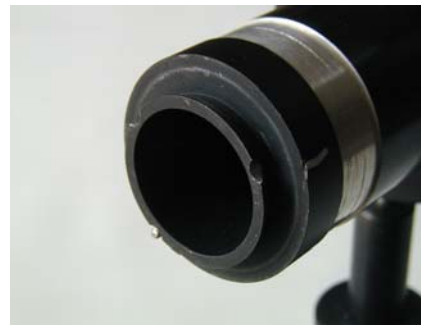
Figure 8 Clamp on an ALI-B tube for accepting an LED.
