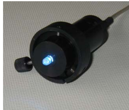
Figure 7 Temperature stabilized LED with built in current stabilizer.
