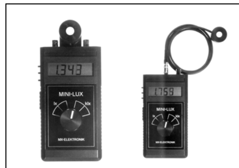
Figure 1 The MINILUX- device with photosensor (silicon-cell with V(\lambda) - and cosine-correction in accordance to DIN 5032, class B).
