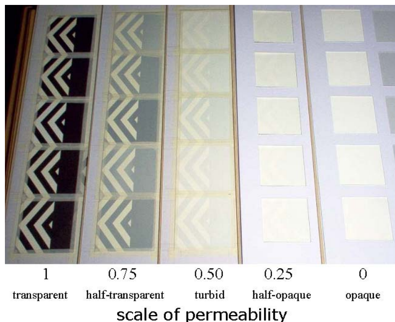
Figure 5. Five steps of permeability. Even when it cannot be appreciated in the photograph, the variation of diffusivity occurs in vertical for each step. With the addition of the variation in darkness, each of these scales originates, in turn, a whole page like the one in Figure 4.
