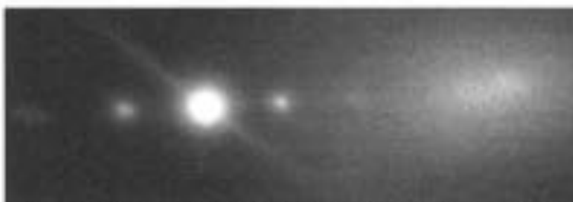
Figure 3. A detailed diffraction pattern produced by the shell of the mollusk Pinctada Margaritifera .
