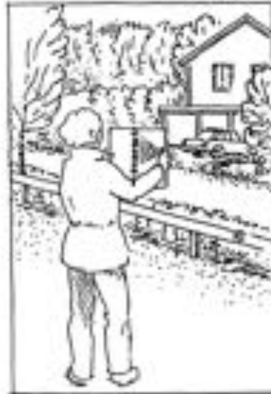
Figure 2: Determination of perceived colour using the NCS atlas.
