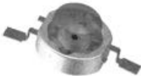
Figure 2: A high output LED, built for several hundred mA drive current.
