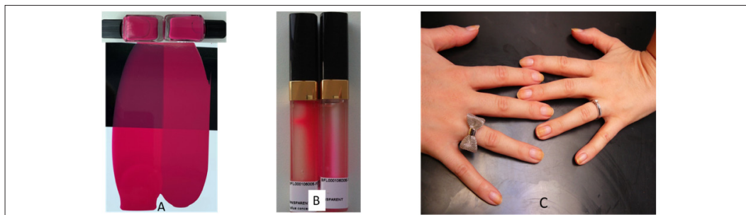
Figure 4: A - Adjustment of nailvarnish opacity. The more transparent nailvarnish contains a quarter of the pigments of the opaquer version (500 microns wet film on contrast card). B - Discoloration of a gloss after 48 hours exposure in a sun test. C - Pigment D&C Red 22 which tints and trace of residual colour on the nails after removing makeup.
