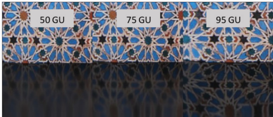
Figure 2: Picture of the three glossiest samples of the black commercial NCS gloss scale.
