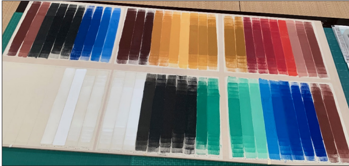
Figure 2: Part of the painted samples. Each sample is painted six layers to ensure the evenness on the surface.
