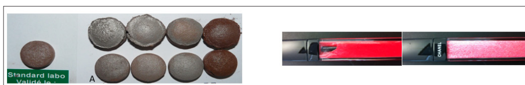
Figure 3: A - Impact of a preservative system on the shade of a baked eyeshadow. B - Impact of the use of D&C Red 30 on lipgloss rheological behavior. Top (left) and bottom (right) faces of a lipgloss stored horizontally.
