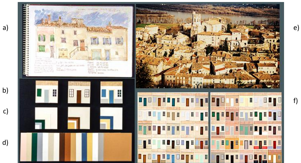
Figure 6: Colour study of Viviers, France: a) watercolour of the situation, with colour notations; b) colour portraits of façades; c) quantitative colour schemes; d) qualitative colour range; e) photograph, general view of the site; f) colour synthesis charts (tableaux de synthèse). Photo: Courtesy Jean-Philippe Lenclos.
