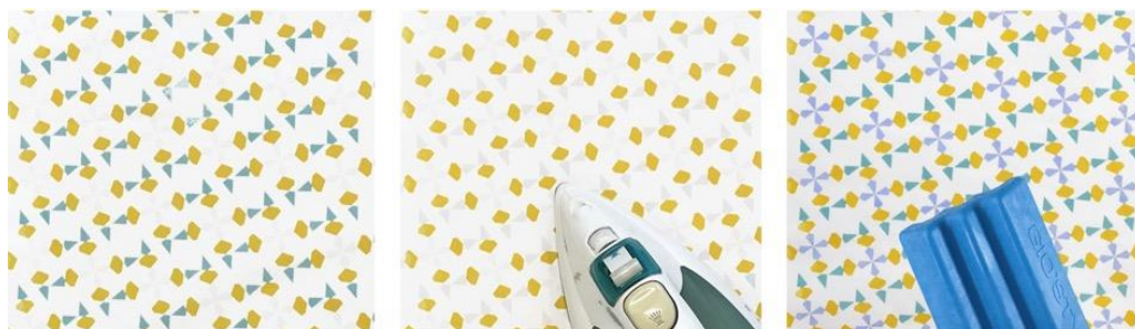
Figure 3, from left to right: The printed fabric produced by inks with activation temperatures 31 and 15°C, the effect at non-heated state, the effect of heating and the effect of cooling the printed fabric.
