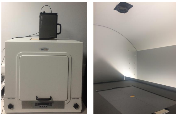
Figure 1: Spectroradiometer setup. On the left side is the outside of the spectrophotometer with the VeriVide DigiEye lighting box, and on the right is the inside of the setup to show the general diffuse/0° geometry of the device.
