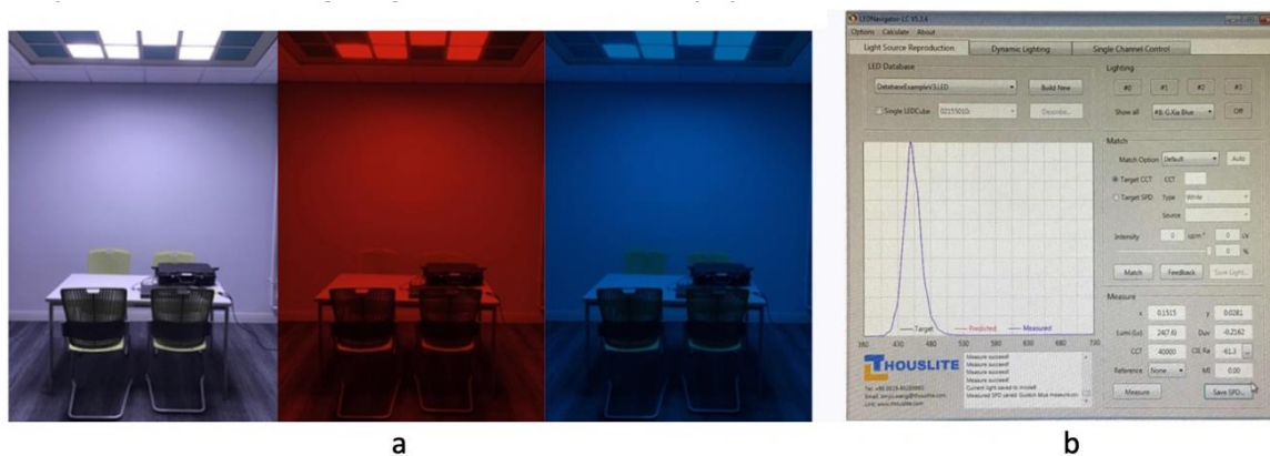
Figure 1: a) The three coloured-lighting conditions in the physical environment. Note that the computer was not in the environments in both physical and VR experiments. b) The interface of Thouslite LED system.
