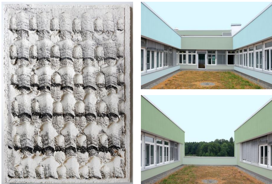
Figure 1: Material sample for simulation of dirt deposit.
