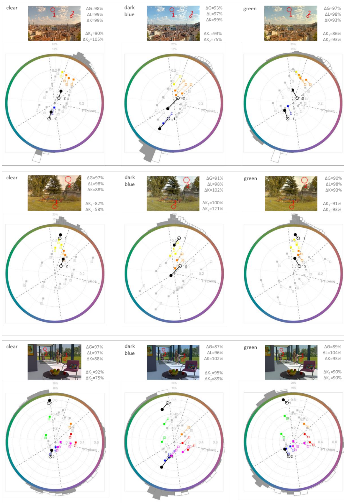
Figure 3: Color shifts predicted by the indicator in the three studied scenes for a clear, a dark blue and a green glass (reference is an ideal window glass of 100% transmission).
