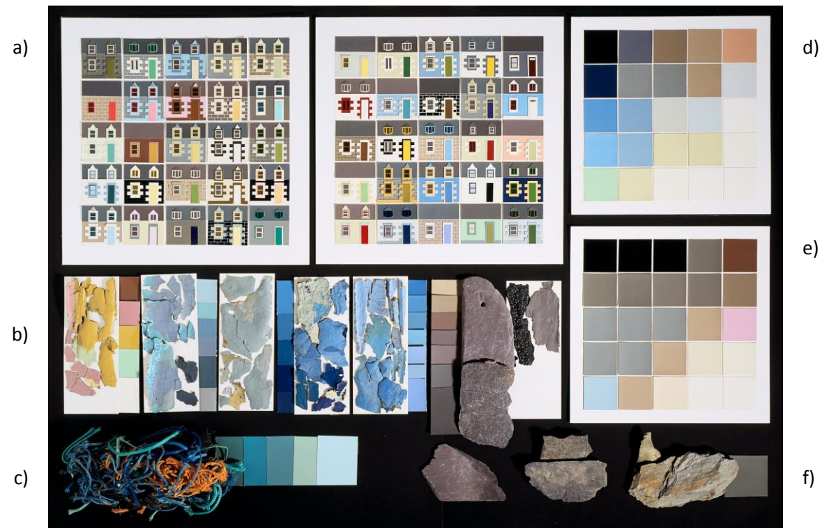
Figure 7: Le Morayshire, Scotland, elements of the analysis and synthesis: a) narrative palettes; b) material samples of the façades, with corresponding colour swatches; c) material samples found on-site, with the colour range of the blues; d), e) general palettes: colours of the façades; f) material samples of the surroundings, with corresponding colour swatches. Photo: Courtesy Jean-Philippe Lenclos.
