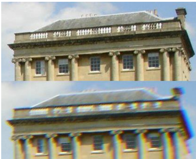
Figure 4: An example withouth chromatic aberration (above) and with chromatic aberration (below).
