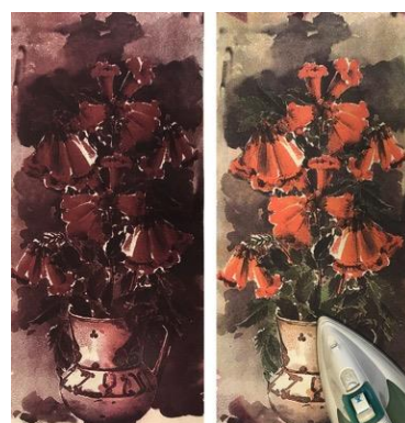
Figure 5, from left to right: The printed fabric produced using four temperature-sensitive colour mixtures consisting of thermochromic inks with activation temperatures of 31°C and static textile pigment pastes, the effect at non-heated state, the effect of heating the printed fabric.
