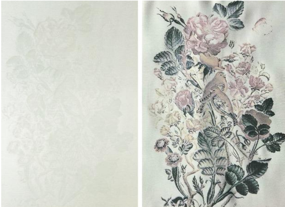
Figure 8: from left to right: the printed fabric produced using photochromic inks overprinted with a layer of black static textile pigment paste, the effect at non-exposed state, the effect of exposing the printed fabric to sunlight.
