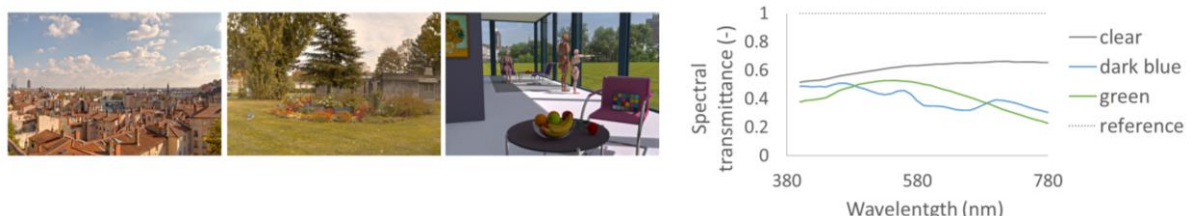
Figure 2: The three studied scenes and the spectral transmittance of the three coated glazing (+ reference).
