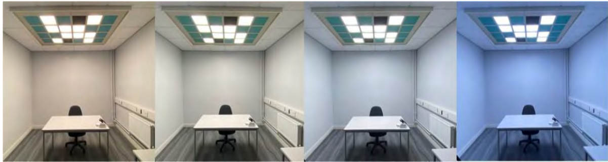
Figure 2. The experimental room with (from left to right) 2500k, 5000k, 8500k, 18500k illumination.
