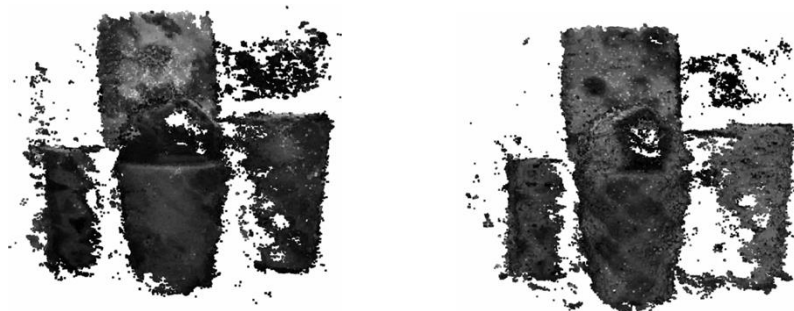
Figure 5. One of the spectral intensities point clouds (left: 430nm, right: 625nm). Compared to the RGB point cloud (Fig. 2), this can represent a 3D point cloud in almost the same range.
