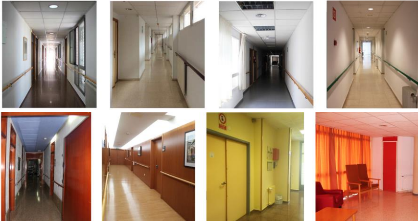
Figure 1: Upper row: Example of public nursing homes' typical corridors in Spain. It is noticeable the presence of dazzles as well as very dark zones. White-coloured spaces with no interest nor stimulus too. Bottom row: Example of chromatic scenes in public nursing homes in Spain. The colours used do not meet any specific design criterion.
