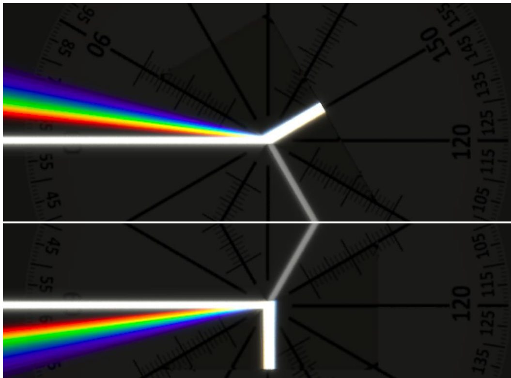
Figure 3: Minimum deviation in Littrow prism (top) and metaprism (bottom).
