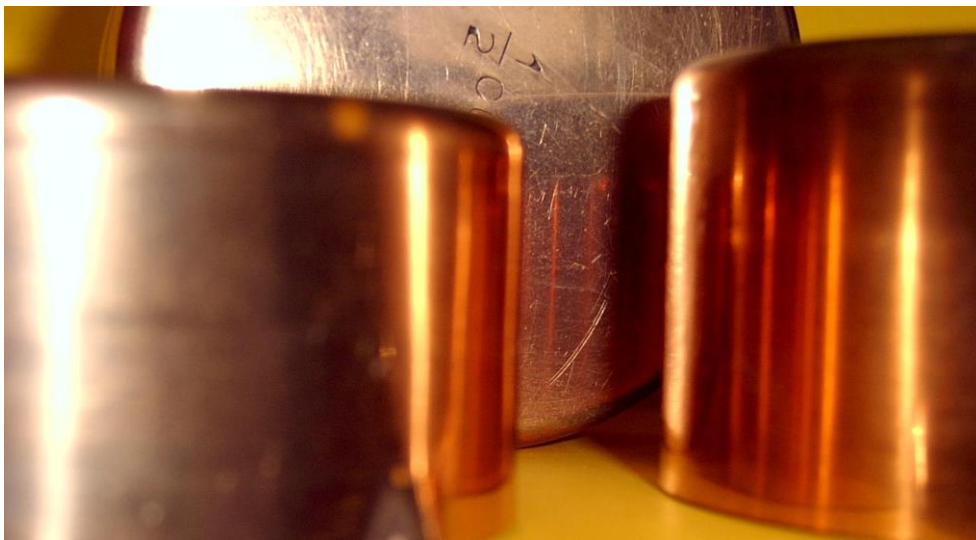
Figure 1: Two metallic surfaces (copper) receiving light and showing the successive images of the specular peak (left) after several mainly specular reflections.
