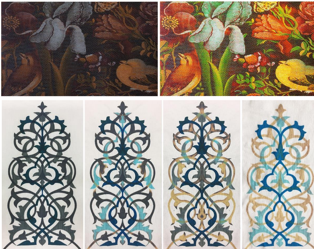
Figure 5: The sample on top consisted of four layers of ink and pigment paste mixtures which are printed on top of one another; that results in a complex dynamic surface pattern with the potential to convey more information in comparison with the simple three colour surface pattern.
