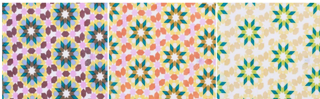
Figure 6: The sample was produced using inks with activation temperatures 27, 37 and 47°C and green static pigment. Fast or slow heating effects the visual expression. Slow heating allows observing the complete range of colour transitions over a longer period of time and in greater detail, e.g. colour changing becomes less intrusive. Here, fast heating becomes more intrusive.
