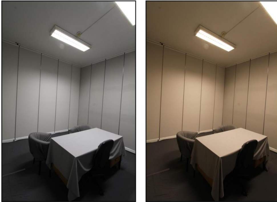
Figure 1: Office Set-up under 4000K (left side) and 2700K (right side) Fluorescent Lighting
