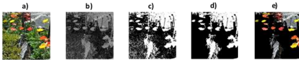
Figure 1: Masking original images with their integrated saliency maps process: (a) original image, (b) integrated saliency map, (c) integrated saliency map segmented, (d) ROI map, and (e) masked image with ROI map.
