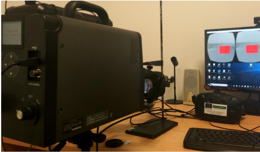
Figure 2: Experimental setup used for chromatic characterization of both HMD.
