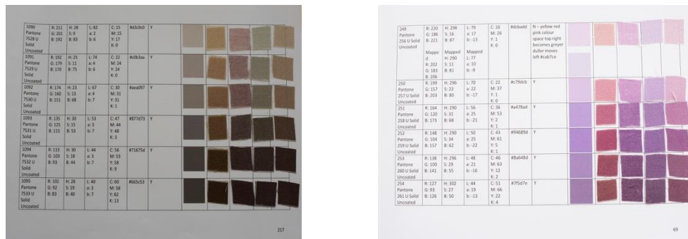
Figure 1: Gooby, B, 2017 Colour Reference Book (Researcher's own collection) Examples of the colour reference book. Each row consists of the digital numeric values (RGB, HSB, Lab, CMYK and Hex) The swatches (left to right) are paper print, wool, linen, cotton and silk.
